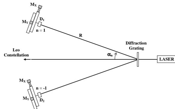
Fig. 1: General layout of the diffraction experiment. Two segmented photo-diodes ( $D_1$  and  $D_2$ ) are positioned using two vertical platforms with two positioning system (micrometers  $M_x - M_y$ ) to detect two diffracted rays produced by a HE-Ne laser on a grating diffraction device. The relative position of a light spot with respect to the center on a segmented photo-diode is obtained by simply measuring the output current of each segment. The setup is mounted on a turntable system
