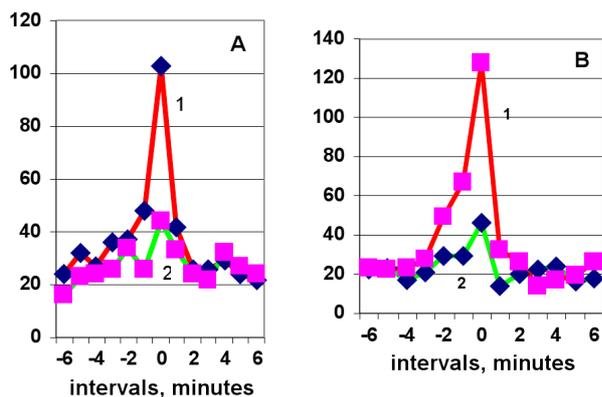
Fig. 2: Palindrome effects in the simultaneous measurements of  $^{239}\text{Pu}$   $\alpha$ -activity with two independent collimator-equipped devices directed East (A) and West (B). Date of measurements, September 22–23, 2003. The axes as in Fig. 1. (A) “East”: (1) “day” versus the following inverse “night”; (2) “day” versus the preceding inverse “night”. (B) “West”: (1) “day” versus the preceding inverse “night”; (2) “day” versus the following inverse “night”.
