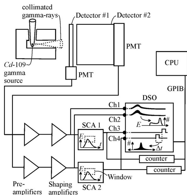
Fig. 3:  $\gamma$ -ray coincidence experiment.
