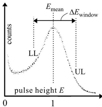
Fig. 1: PMT pulse-height response. Data according to [16].
