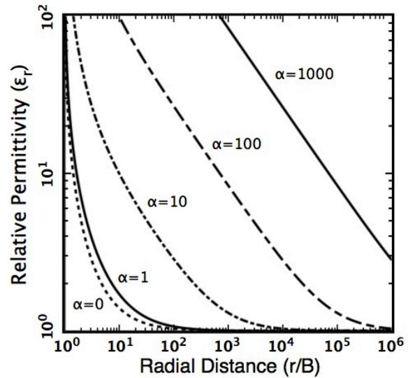
Fig. 2: The relative permittivity  $\epsilon_r$  or the electric field ratio  $E_C/E$  versus the normalized radial distance  $r/B$  for a charged object with  $\alpha = 0, 1, 10, 100, 1000$ , respectively.
